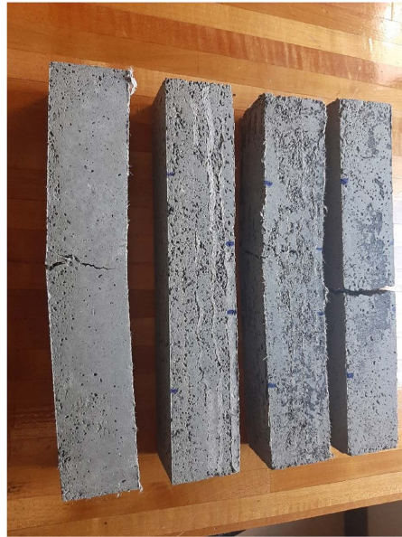
Figure 15. Failure and fracture patterns of all treatment types.
