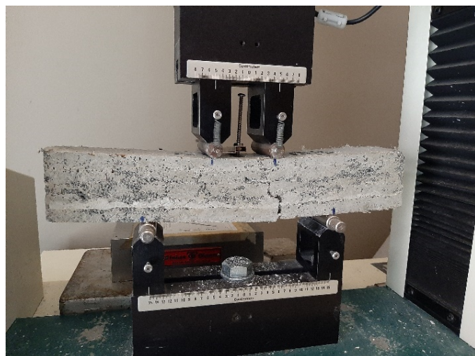
Figure 14. Failure pattern of L-F samples.
