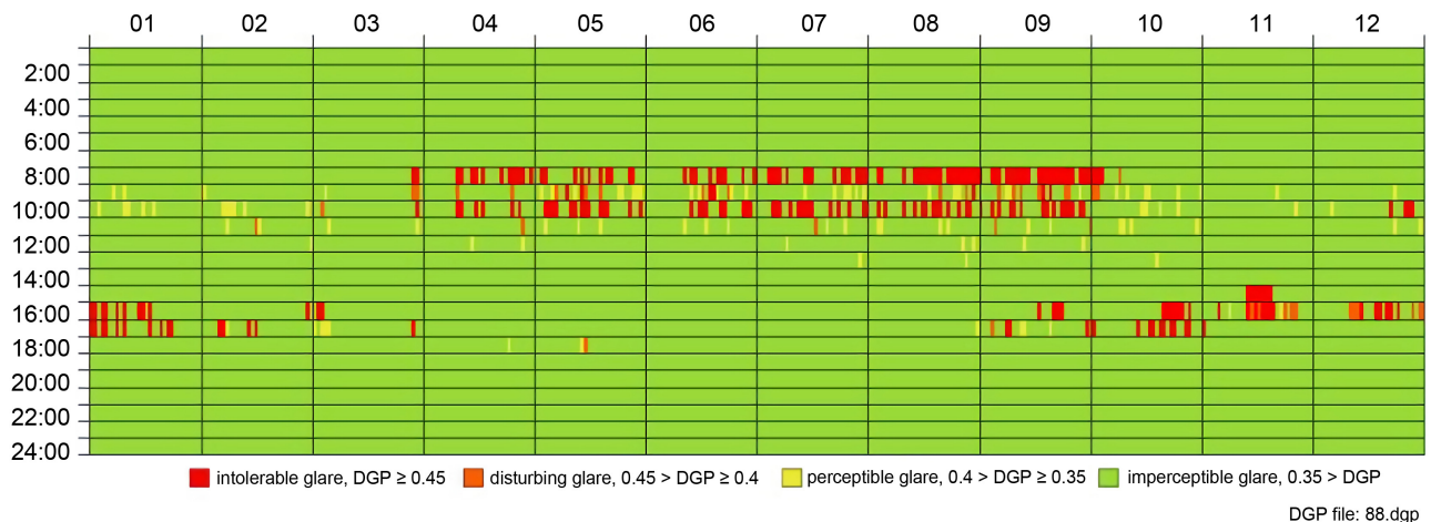
Figure 34. Daylight glare probability of single panel glazing with 88% VT.
