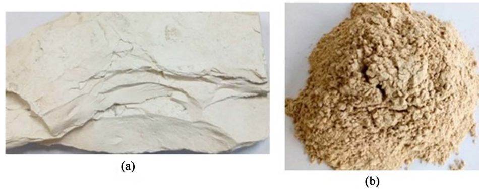
Figure 2. (a) Attapulgite in its natural state; (b) Attapulgite in its crushed and calcined state.
