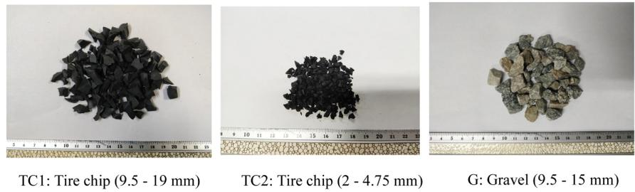
**Figure 4.** Tire chips and gravel used in the preparation of GTCM sample.
