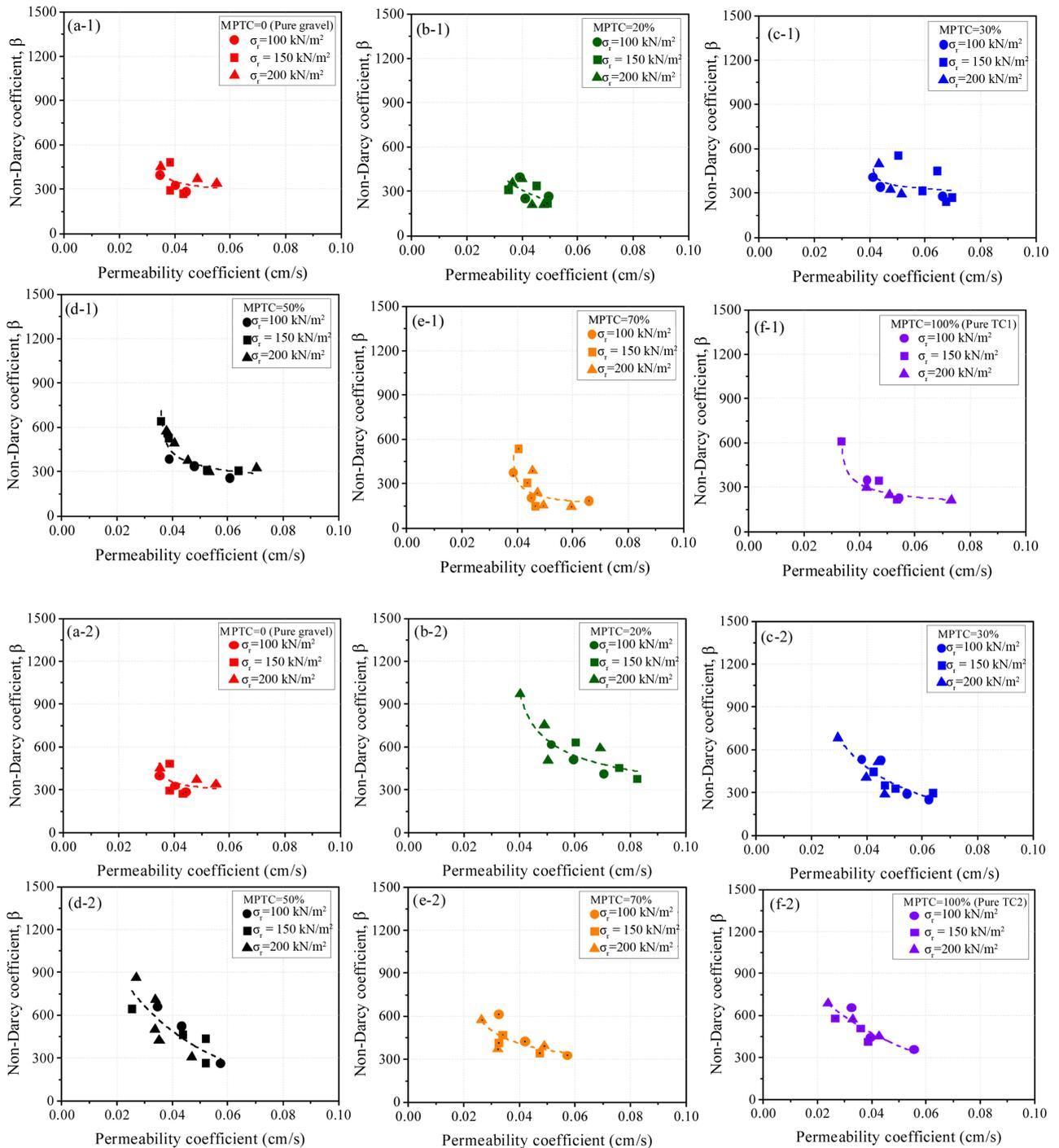
**Figure 12.** Relationship between permeability coefficient  $k$  and non-Darcy coefficient  $\beta$ . TC1G: (a-1) MPTC = 0; (b-1) MPTC = 20%; (c-1) MPTC = 30%; (d-1) MPTC = 50%; (e-1) MPTC = 70%; (f-1) MPTC = 100%. TC2G: (a-2) MPTC = 0; (b-2) MPTC = 20%; (c-2) MPTC = 30%; (d-2) MPTC = 50%; (e-2) MPTC = 70%; (f-2) MPTC = 100%.
