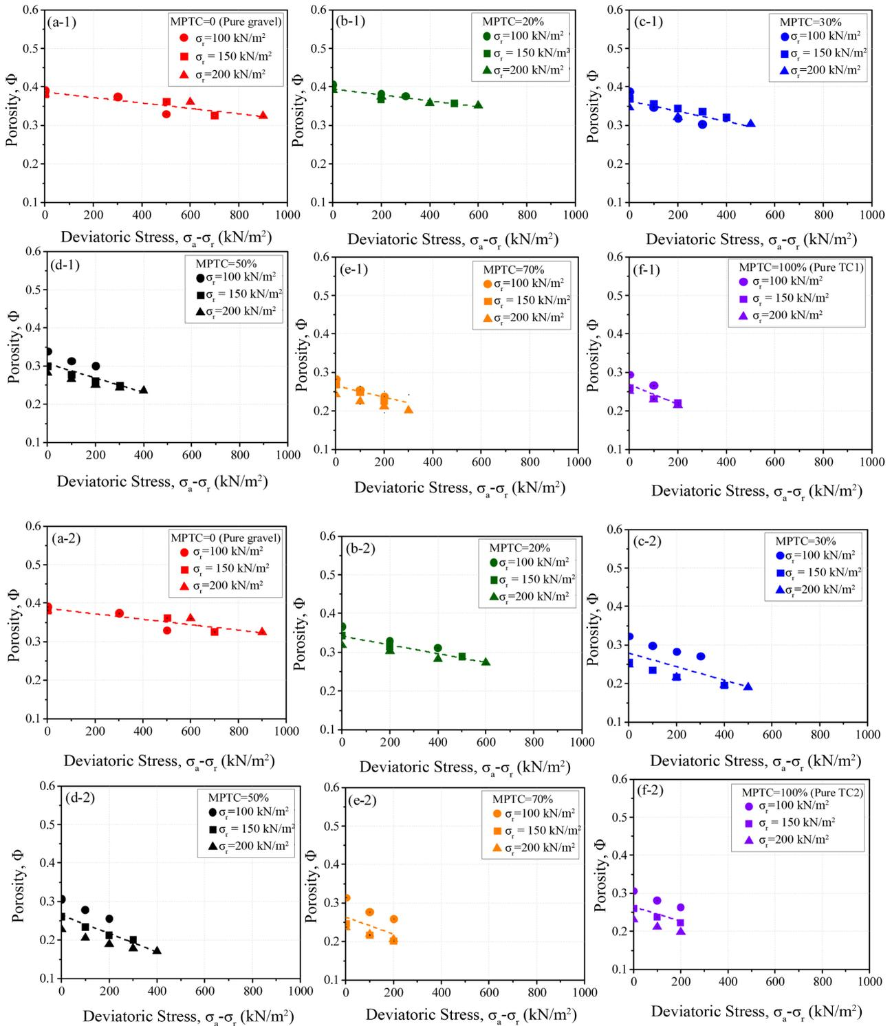
**Figure 10.** Variation of porosity during axial compression. TC1G: (a-1) MPPTC = 0; (b-1) MPPTC = 20%; (c-1) MPPTC = 30%; (d-1) MPPTC = 50%; (e-1) MPPTC = 70%; (f-1) MPPTC = 100%. TC2G: (a-2) MPPTC = 0; (b-2) MPPTC = 20%; (c-2) MPPTC = 30%; (d-2) MPPTC = 50%; (e-2) MPPTC = 70%; (f-2) MPPTC = 100%. TC1: 9.5 - 19 mm; TC2: 2 - 4.75 mm; G: 9.5 - 15 mm.
