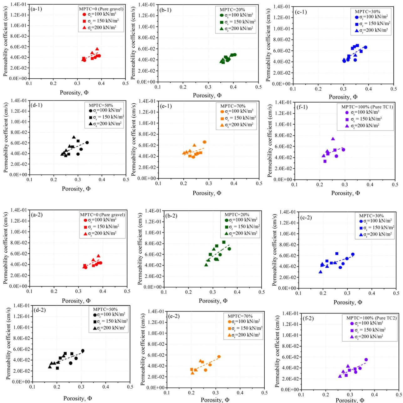
**Figure 11.** Relationship between porosity  $\Phi$  and permeability coefficient  $k$ . TC1G: (a-1) MPTC = 0; (b-1) MPTC = 20%; (c-1) MPTC = 30%; (d-1) MPTC = 50%; (e-1) MPTC = 70%; (f-1) MPTC = 100%. TC2G: (a-2) MPTC = 0; (b-2) MPTC = 20%; (c-2) MPTC = 30%; (d-2) MPTC = 50%; (e-2) MPTC = 70%; (f-2) MPTC = 100%.
