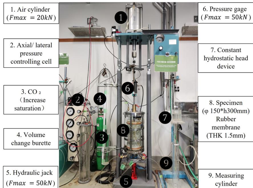
**Figure 7.** Large-scale triaxial compression and permeability testing system.
