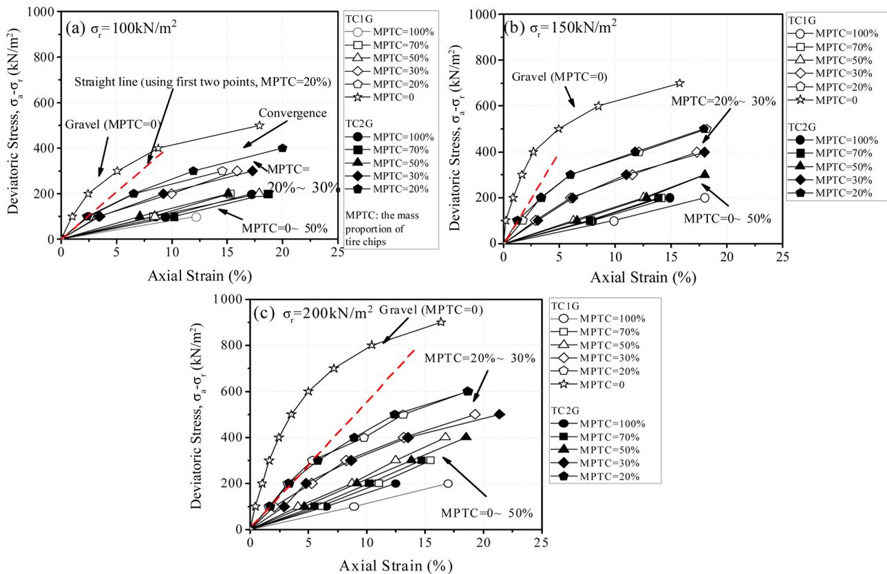
**Figure 8.** Effect of MPTC (mass proportion of tire chips) on deviatoric stress-axial strain. (a)  $\sigma_r = 100 \text{ kN/m}^2$ ; (b)  $\sigma_r = 150 \text{ kN/m}^2$ ; (c)  $\sigma_r = 200 \text{ kN/m}^2$ .
