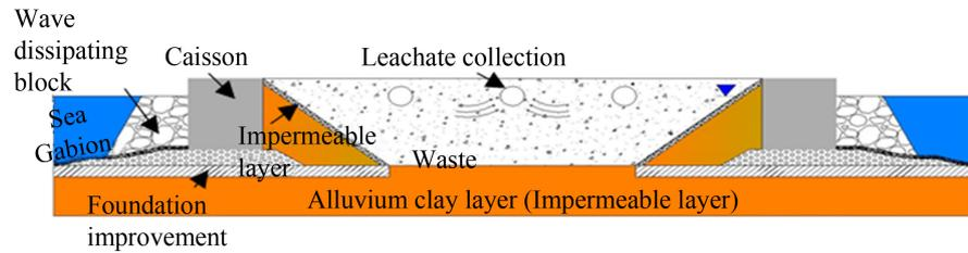
**Figure 1.** Marine landfill drainage system.
