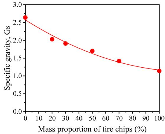
**Figure 5.** Specific gravity of GTCM particles.
