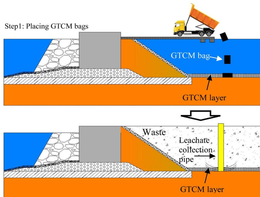
**Figure 3.** Marine landfill with a GTCM reinforcement layer.
