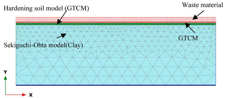
**Figure 13.** Finite element model of the reinforced case.
