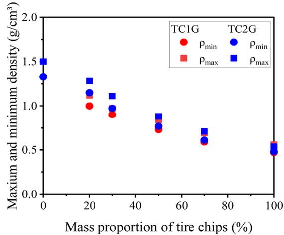
**Figure 6.** Maximum and minimum densities of GTCM particles.
