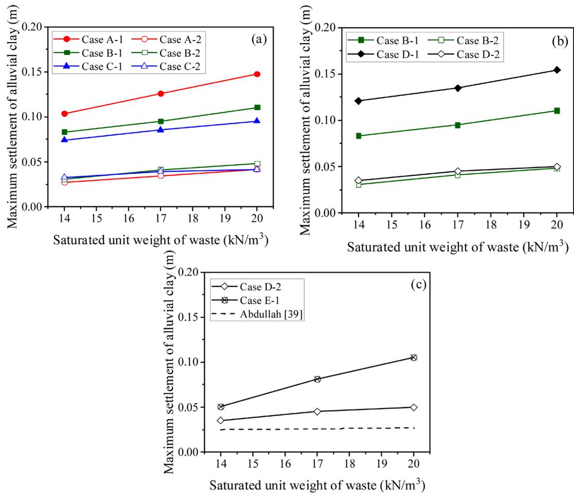
**Figure 14.** Maximum settlement of alluvium clay with different (a) clay thicknesses (b) clay widths (c) materials.
