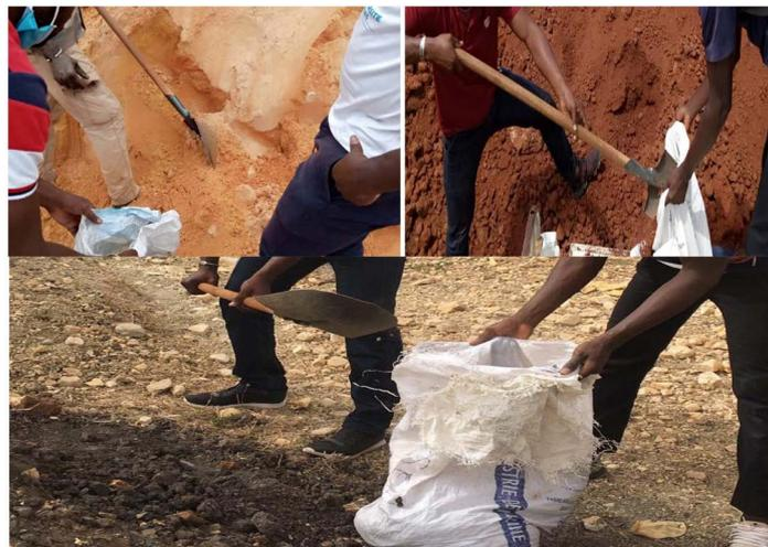
**Figure 1.** Collecting samples of sand (left), laterite (right) and clay (bottom).
