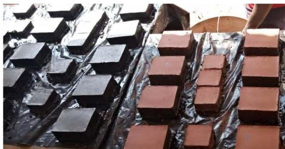
**Figure 3.** Clay bricks (left) and laterite bricks (right).
