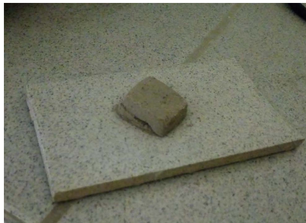
Plate 2. Sample of ceramics before loading into the XRF unit.
