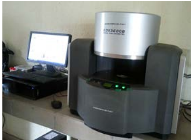
Plate 1. EDX3600B EDXRF spectrometer machine.
