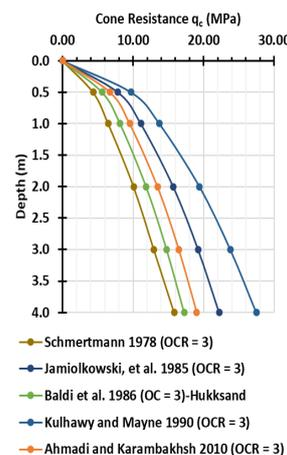
**Figure 3.**  $q_c$  profile based on over consolidation ratio (OCR = 3).
