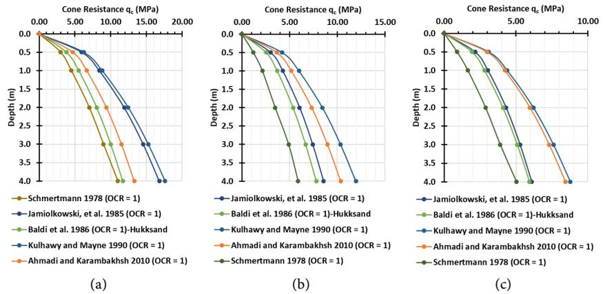
Figure 4.  $q_c$  profile for Normally consolidated sands. (a)  $D_r = 85\%$ ; (b)  $D_r = 70\%$ ; (c)  $D_r = 60\%$ .
