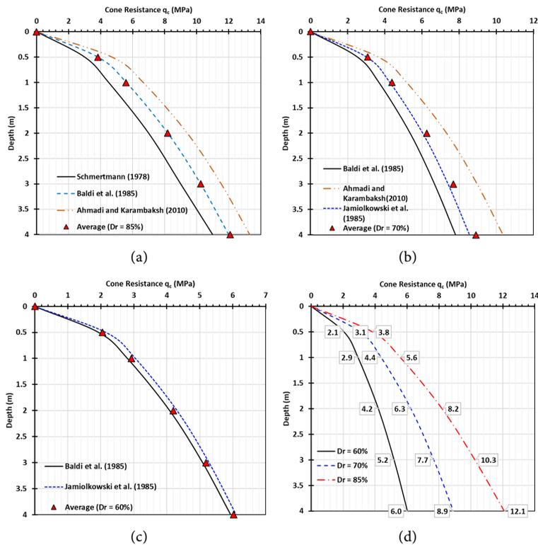
Figure 5. Recommended  $q_c$  performance line based on sand relative density. (a)  $q_c$ -profile for  $D_r = 85\%$ ; (b)  $q_c$ -profile for  $D_r = 70\%$ ; (c)  $q_c$ -profile for  $D_r = 60\%$ ; (d) Average  $q_c$ -profiles.
