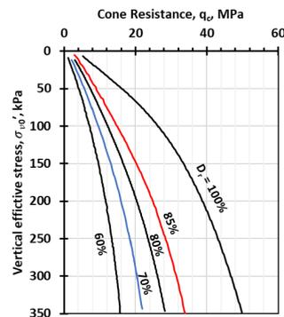
**Figure 1.** Cone tip resistance as a function of overburden pressure and soil relative density (after [14]).
