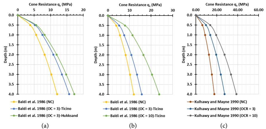
**Figure 2.** Effect of over consolidation ratio on the cone tip resistance performance line. (a) Effect of sand type on the value of  $q_c$ ; (b) Variation of OCR from [3]; (c) Variation of OCR from [20].
