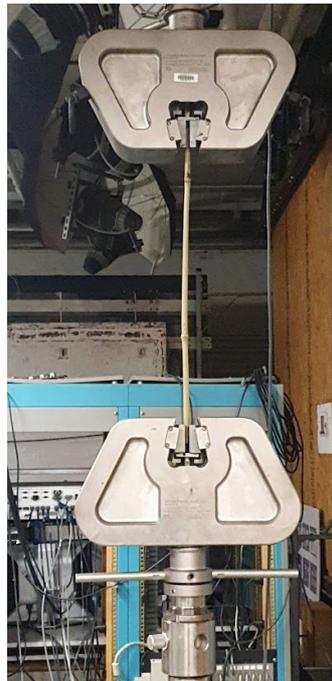
**Figure 7.** Testing bamboo's tensile strength in a universal testing machine.
