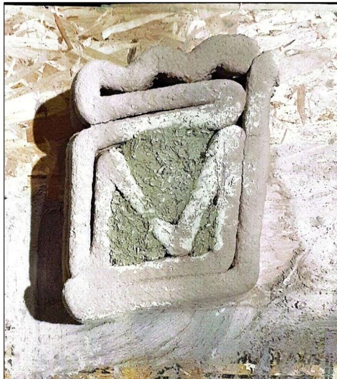
**Figure 10.** 3D printed cobcrete specimen with embedded hempcrete fillers in the void cells.
