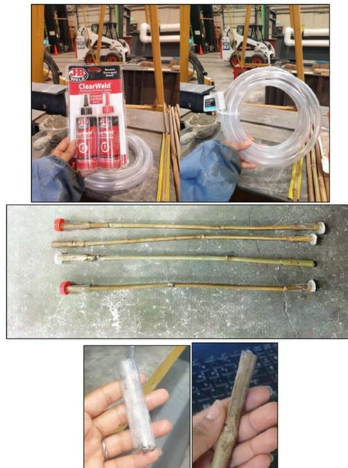
**Figure 3.** Epoxying bamboo on a plastic pipe.
