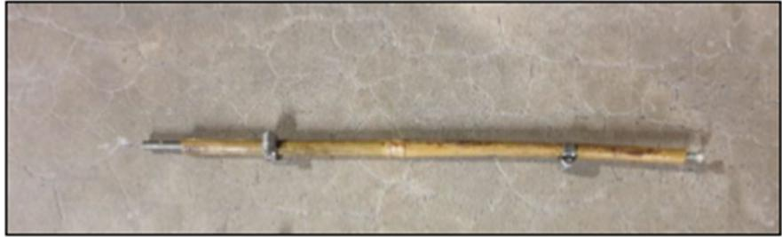
**Figure 6.** Inserting extended steel rod and hose clamping bamboo tips.
