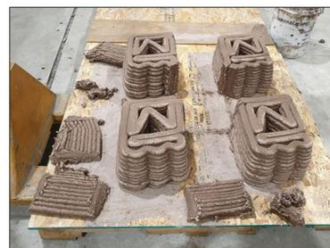
Separated four sections of cobcrete wall pieces by eliminating the connecting wall toolpath before it fully hardened
