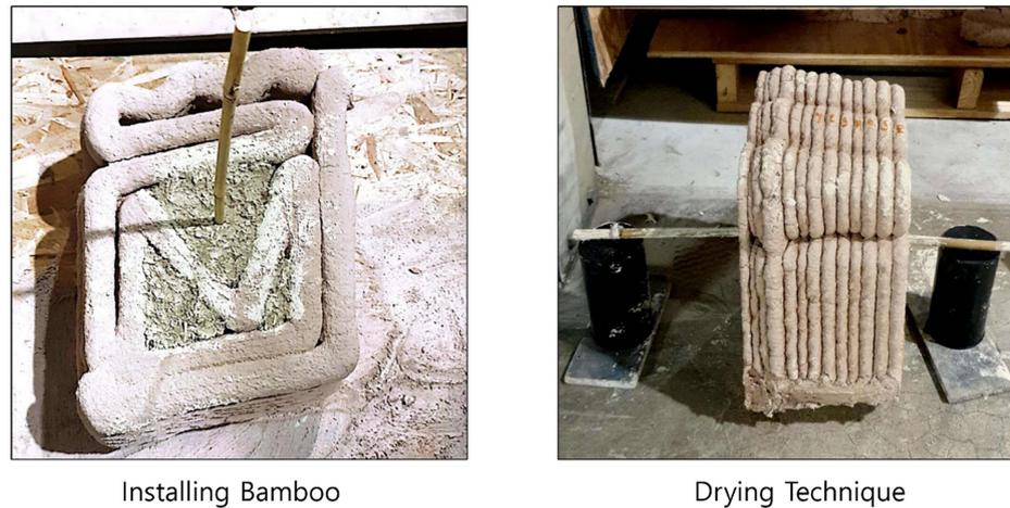
**Figure 11.** Bamboo installation and drying technique.
