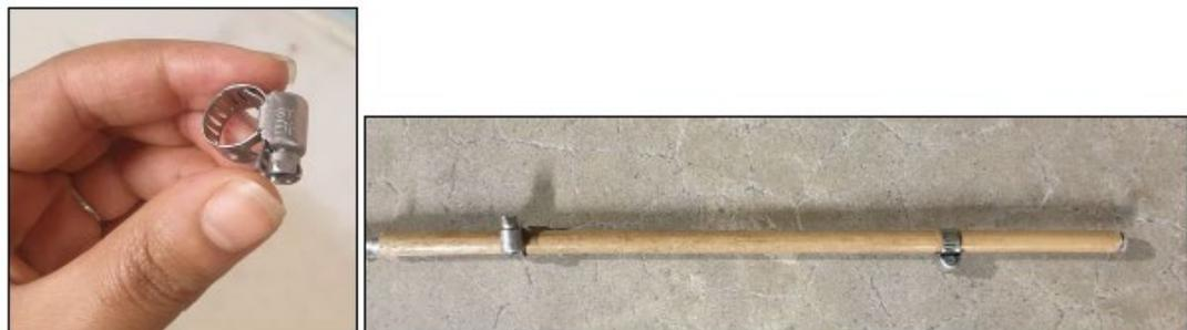
**Figure 5.** Inserting steel rod and hose clamping bamboo tips.
