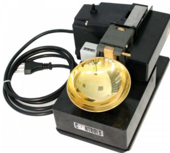
**Figure 3.** Casagrande device.
