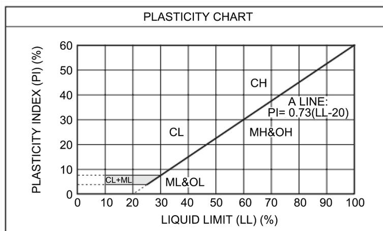
**Figure 10.** Soil Plasticity chart as per Unified soil classification system.
