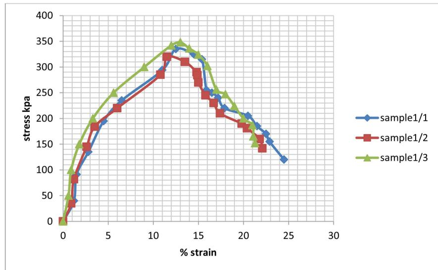
**Figure 14.** Stress and axial strain as measured on the three different samples of Soil 1.
