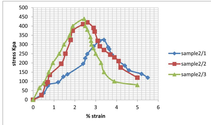
**Figure 15.** Stress and axial strain as measured on the three different samples of Soil 2.
