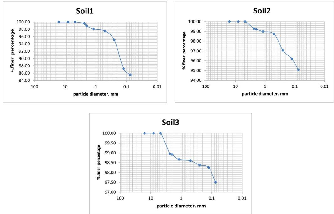
Figure 11. Particle size distributions charts of the three soils used in this study.
