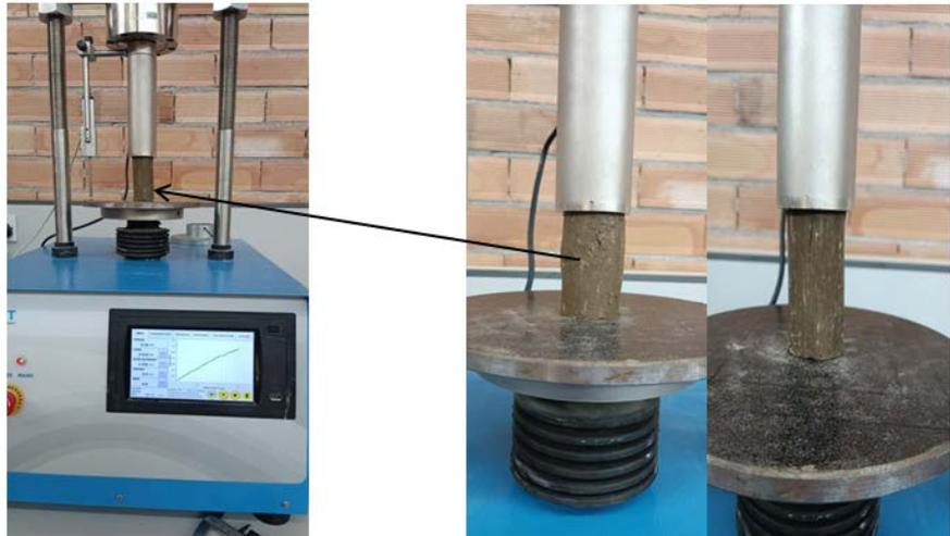
**Figure 8.** (a) Soil sample being tested using an unconfined compressive strength testing machine; (b) Unconfined compression test of soil sample under pressure.
