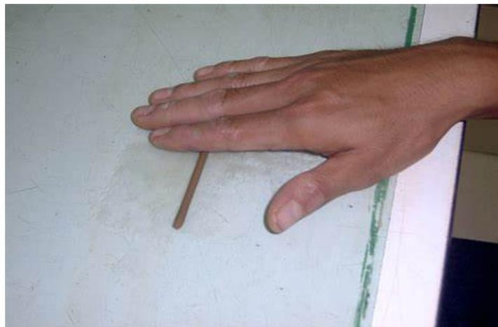
**Figure 4.** Plastic limit test.
