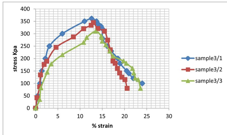
**Figure 16.** Stress and axial strain as measured on the three different samples of Soil 3.
