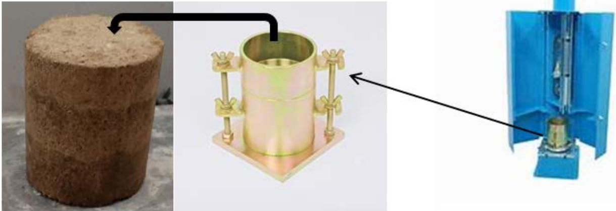
**Figure 7.** Compaction test mould and automatic soil compactor.
