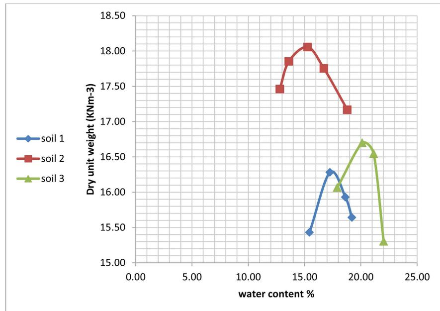
**Figure 13.** Compaction curves for soil samples showing the typical behaviour of an optimum moisture content (OMC) where the dry density is maximised.
