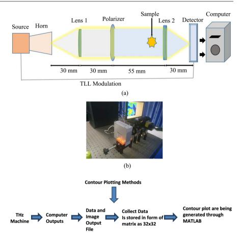
**Figure 1.** Details THz optical setup with a working function. (a) Optical THz setup with complete working processes; (b) THz hardware setup with complete working processes.
