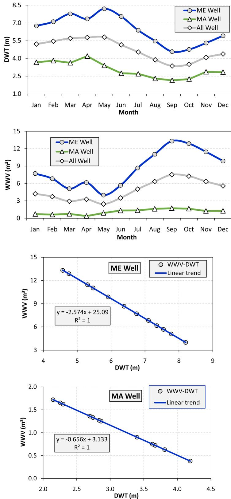
**Figure 3.** Time-series plots of monthly Depth to Water Table (DWT) and Well Water Volume (WWV) and the corresponding correlations for manually dug (ME) and mechanically drilled (MA) wells in the study area.
