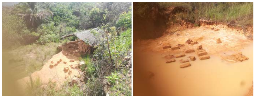
Figure 5. Production area for blocks of unstabilised earth (adobe). West Cameroon.
