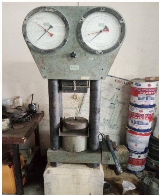
Figure 10. Mould and the hydraulic press used for the manufacture of the specimens.
