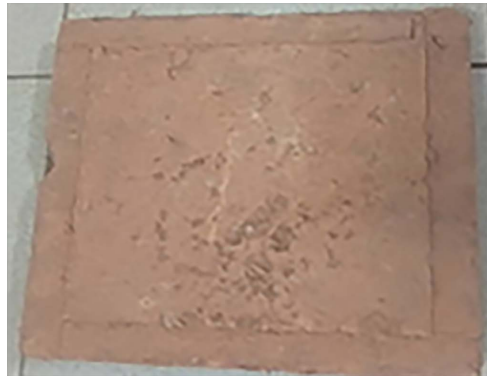
Figure 2. Sample brick for thermal conductivity testing.
