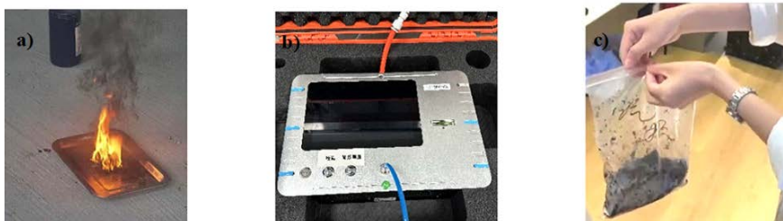
Figure 2. fire debris sample measurement, (a) material is doused with an accelerant and ignited and then extinguished with water, (b) an air background is collected from the burn area, and (c) the vapors from fire debris sample enclosed in a bag is opened and measured.
