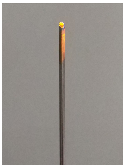
Figure 9. The photo of the fluorescence optical fiber probe.
