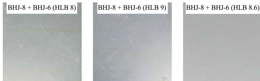
Figure 6. Effect of compound inversion agent on an aqueous solution of drag reducer emulsion.
