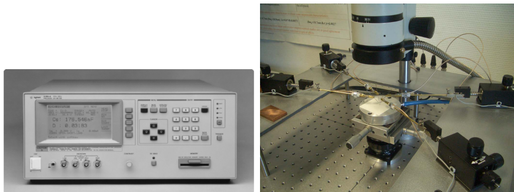
Figure 3. Low frequency measuring equipment: LCRmeter and Four-point tester [7].
