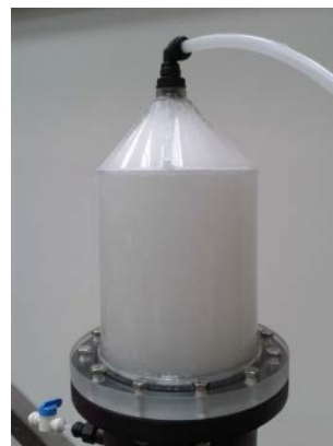
Figure 4. Column in extraction phase after addition of MIBC.
