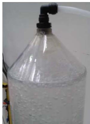
Figure 6. Column in extraction phase after addition of casein.
