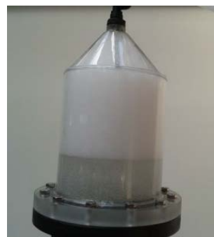
Figure 5. Column in extraction phase after addition of Tween 20.
