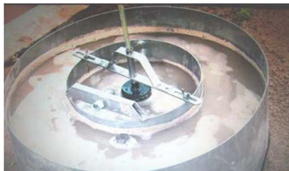
Figure 3. Double ring infiltrometer Source [9]
