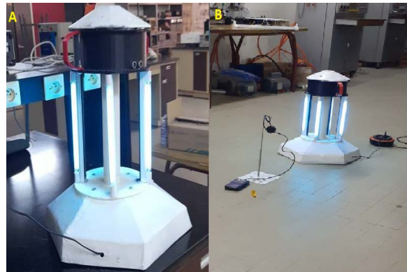
Figure 1. UVGI. A: Automated UV-C device photo; B: irradiation intensity measurements set up.
