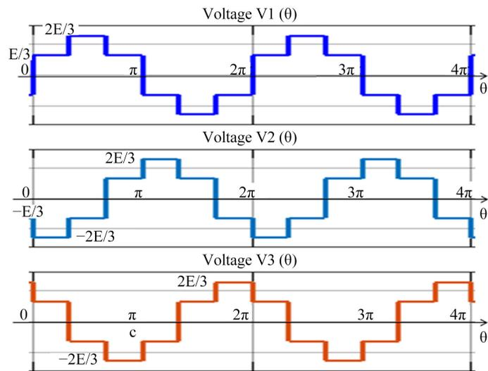
Figure 3. Voltage signals  $V_1(\theta)$ ,  $V_2(\theta)$  and  $V_3(\theta)$ .
