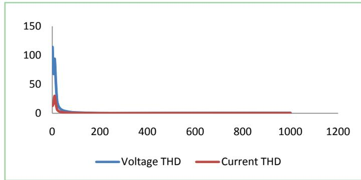
**Figure 5.** THD of voltage and current as a function of  $q \times C_{max}$ ;  $q \in [1;1000]$ .
