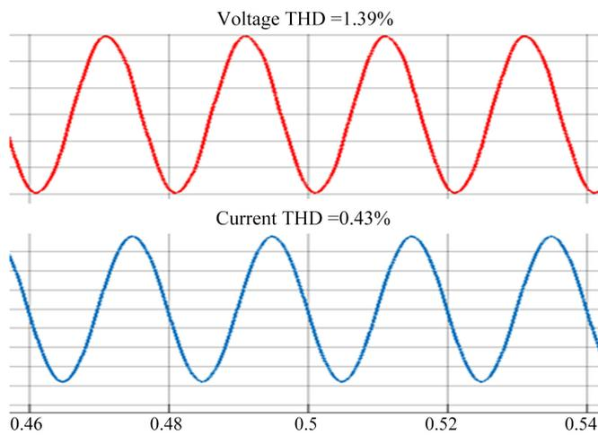
Figure 13. Voltage and current waveforms for  $L = L_{maxi}$  and  $C = 100 \times C_0$ .
