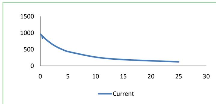
**Figure 10.** RMS current as a function of  $q \times L_{max}$ ;  $q \in [0.01; 25]$ .
