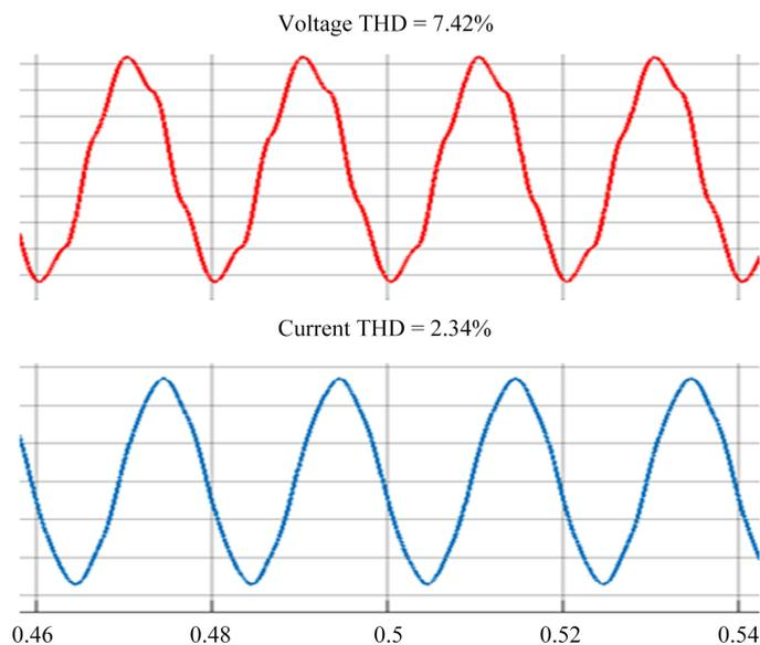
**Figure 11.** Voltage and current waveforms for  $L = L_{max}$  and  $C = 35 \times C_0$ .
