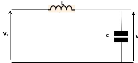
**Figure 1.** Single phase filter circuit ( $L$ - $C$ ).
