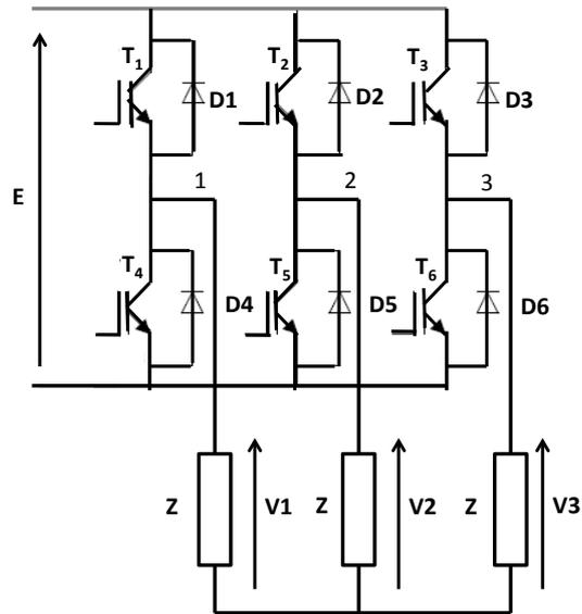
Figure 2. Three-phase inverter.
