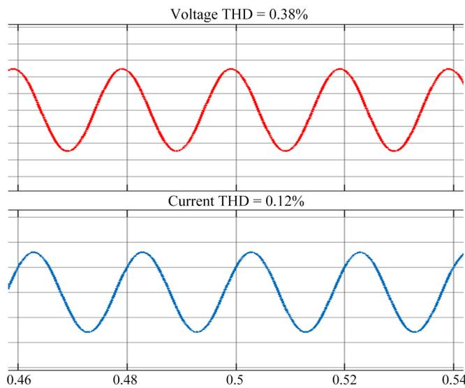
Figure 14. Voltage and current waveforms for  $L = L_{maxi}$  and  $C = 400 \times C_0$ .
