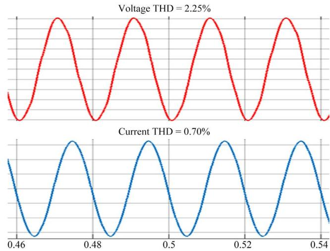
Figure 12. Voltage and current waveforms for  $L = L_{maxi}$  and  $C = 75 \times C_0$ .
