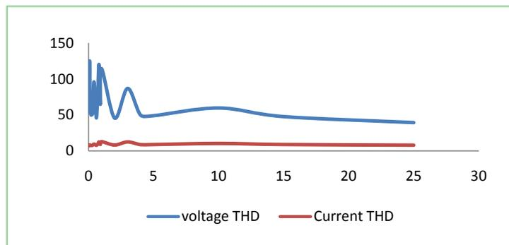
**Figure 8.** THD of voltage and current as a function of  $q \times L_{max}$ ;  $q \in [0.01;25]$ .
