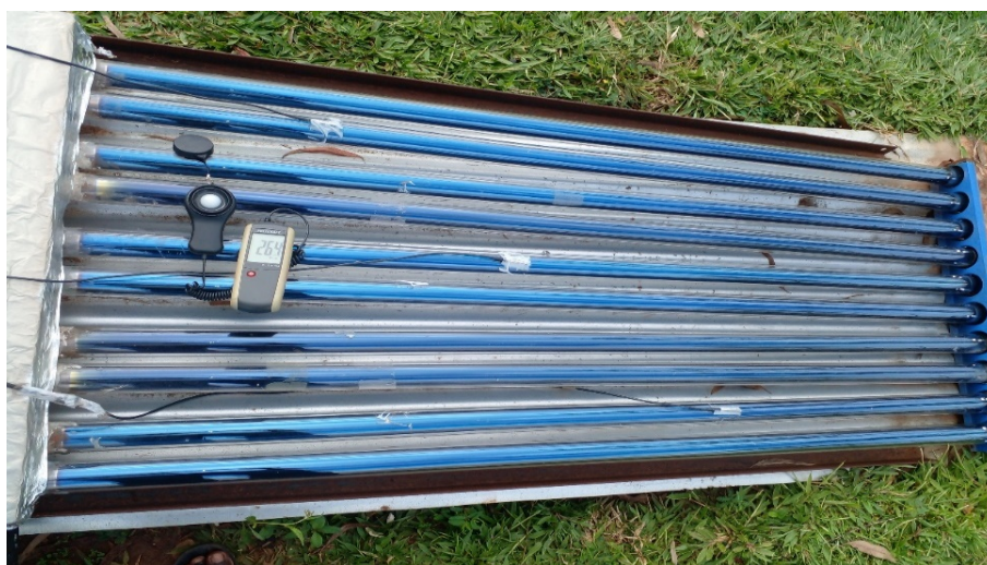
Figure 4. Designed evacuated tube solar collector view.
