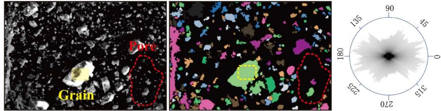
**Figure 8.** SEM image, binary image and particle distribution direction of BNS133 sample.
