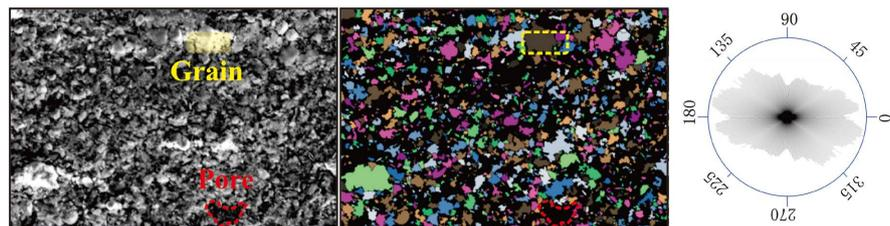
**Figure 11.** SEM image, binary image and particle distribution direction of BNS167 sample.
