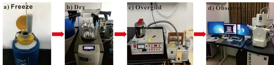
**Figure 5.** Scanning electron microscope test process.
