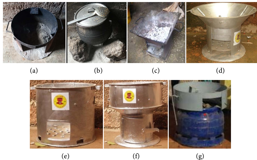
Figure 2. Cookstoves used by households in the city of Ouagadougou. (a) Traditionnal metallic cookstove (malgasian wood cookstove); (b) Traditionnal Three-stone cookstove; (c) Traditionnal metallic cookstove (malgasian charcoal stove); (d) Multipot sizes cookstove; (e) Ouaga métallique cookstove; (f) Burkina mixte cookstove; (g) Faitout Gas cookstove.
