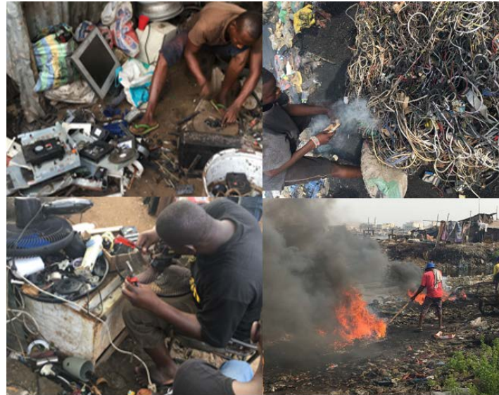
Figure 4. Dismantle and incineration of e-waste in Cotonou workshops which exemplifies the work conditions, notably that activities are generally performed on the bare group and without personal protections.
