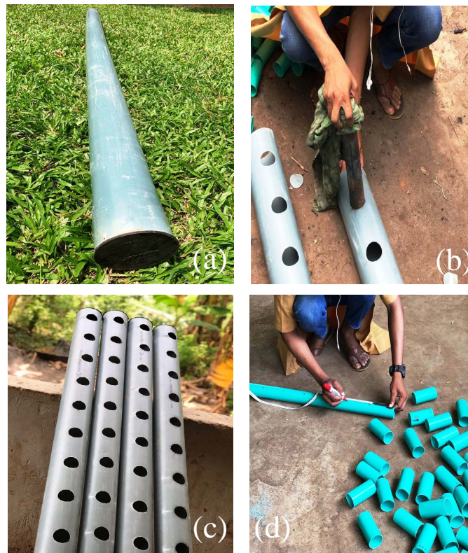
Figure 1. (a) 10 cm diameter Pipe at initial stage, (b) Marking of 5 cm diameter holes on the 10 cm diameter pipe at 15 cm interval with a hot 5 cm diameter galvanized iron pipe, (c) 10 cm diameter underground reservoir pipes perforated in definite spacing of 15 cm apart, (d) Marking and cutting of the capillary pipes (10 cm long and 5 cm diameter).
