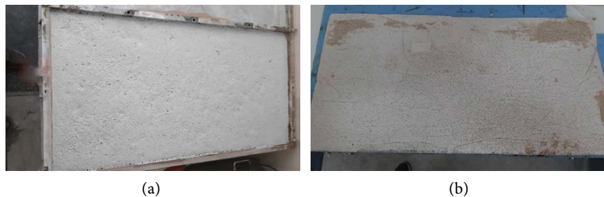
Figure 2. Samples from the large scale in situ production of the screed for further testing of the material.
