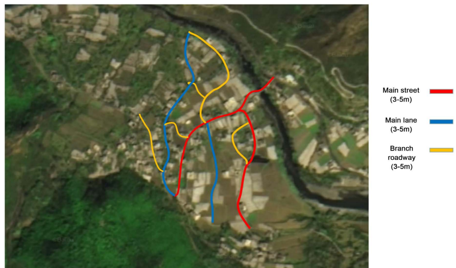
Figure 4. Schematic diagram of main traffic layout in Dasang Village.
