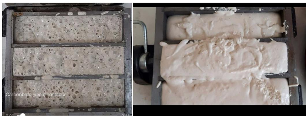
**Figure 6.** Effect of surfactant addition. Right picture geopolymer with 0.2%w/w surfactant, left no surfactant.
