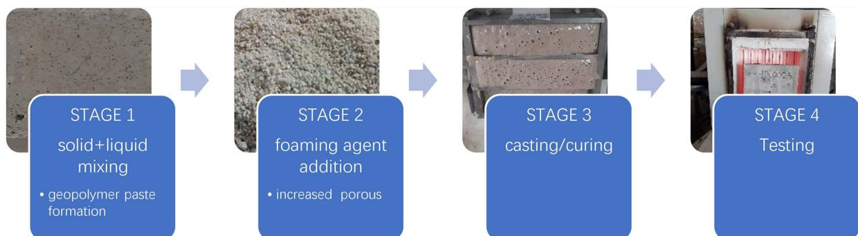
Figure 3. Foamed geopolymer production steps.
