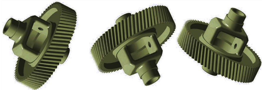
Figure 3. Model after reduction of the web thickness.
