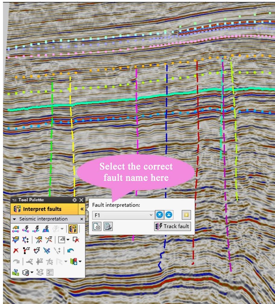
Figure 4. Fracture manual interpretation interface.
