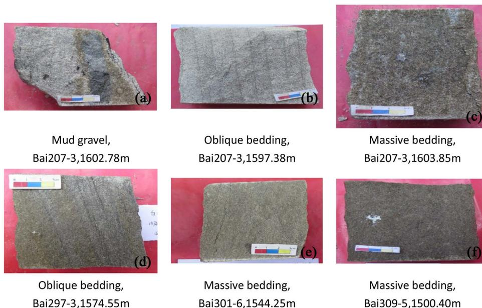
**Figure 2.** Typical core photos of Yan10 member of Bai211 area.
