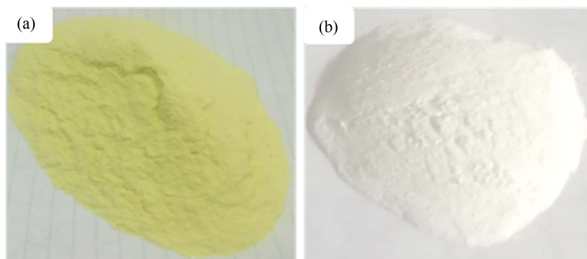
Figure 3. Zircon opening products; (a) ZrOCl_2 and (b) ZrO_2 powder.
