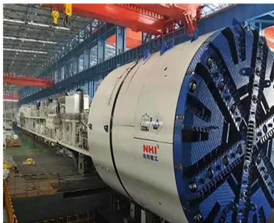
Figure 4. Shield tunneling machine.
