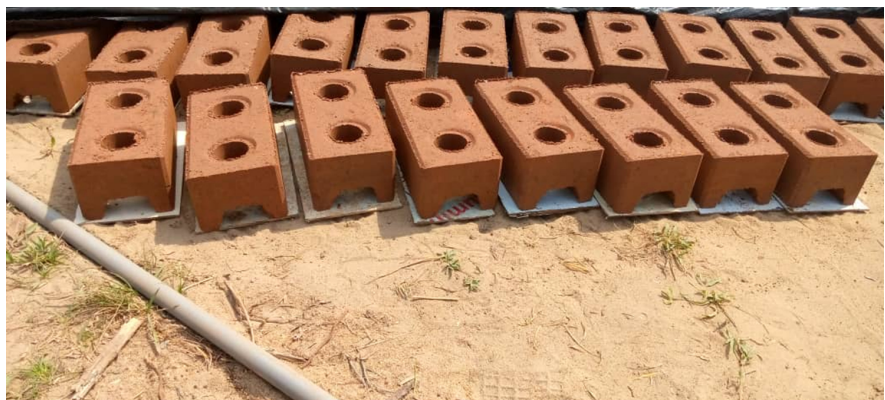
Figure 4. Stabilized interlocking clay bricks newly made.
