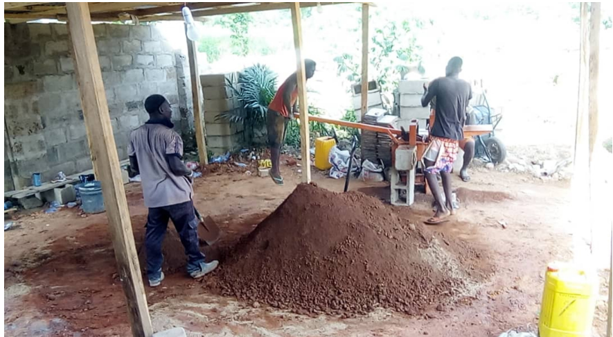
Figure 6. The manufacturing process of stabilized interlocking clay bricks.
