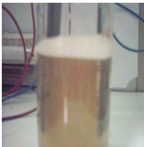
Figure 5. White froth formation at the surface of solution during EC application.
