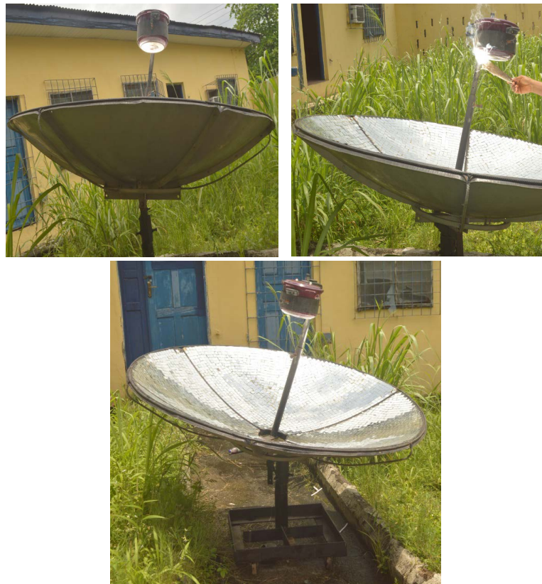
Figure 7. Domestic solar cooker in operation.
