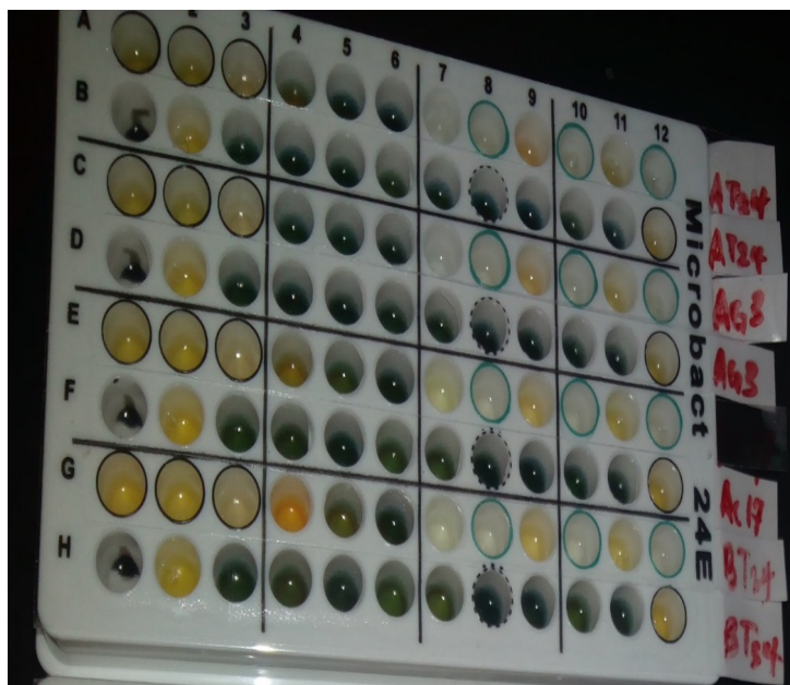
Figure 1. Microbact™ GNB 24E kit after the addition of bacterial suspension in each well before incubation.
