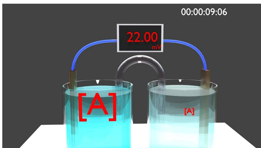
**Figure 1.** Example of an electrochemical cell. There is a potential because there are chemical reactions at the interfaces and the compartments are connected to each other by an external electric circuit and an ionic circuit is thus created in the electrolytes.
