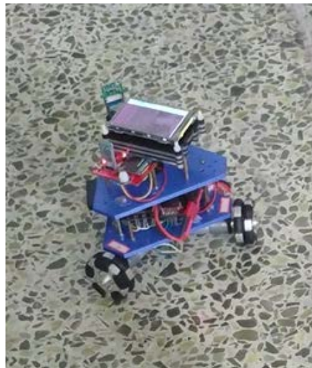
Figure 6. Omni-wheel moving platform test.
