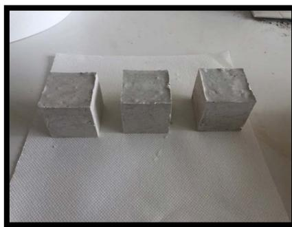
**Figure 3.** Glass based geopolymer.
