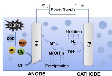
Figure 1. The schematic of an EC cell with DBP formation [1].
