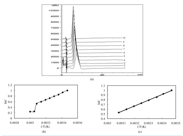
Figure 4. Effect of column temperature on the retention of HP-β-CD. (a) 1—15°C, 2—20°C, 3—25°C, 4—30°C, 5—35°C, 6—40°C, 7—45°C, 8—50°C, 9—55°C, 10—60°C. (b) Plot of ln k' versus the column temperature in the range of 15°C - 60°C. (c) Plot of ln k' versus the column temperature in the range of 15°C - 50°C, R² > 0.99. Mobile phase: acetonitrile/water (80/20, v/v). Flow rate: 1.5 mL/min. Sample: HP-β-CD (3.0 mg/mL) dissolved in the mobile phase. Injection volume: 20 μL.
