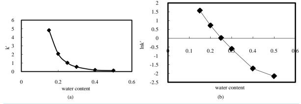
Figure 2. (a) Plot of retention factor (k') versus the content of water in the mobile phase. (b) Plot of  $\ln k'$  versus the content of water in the mobile phase. Column temperature: 35°C. Flow rate: 1.5 mL/min. Sample: HP-β-CD (3.0 mg/mL) dissolved in the mobile phase. Injection volume: 20 μL.
