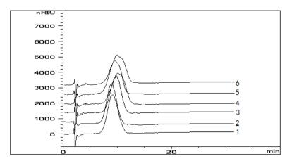
**Figure 3.** Chromatograms at different pH: 1—pH = 3.0, 2—pH = 4.0, 3—pH = 5.0, 4—pH = 5.5, 5—pH =6.0, 6—pH = 6.5. Column temperature: 35°C. Mobile phase: acetonitrile/water with buffer (80/20, v/v). Flow rate: 1.5 mL/min. Sample: HP- $\beta$ -CD (3.0 mg/mL) dissolved in the mobile phase. Injection volume: 20  $\mu$ L.
