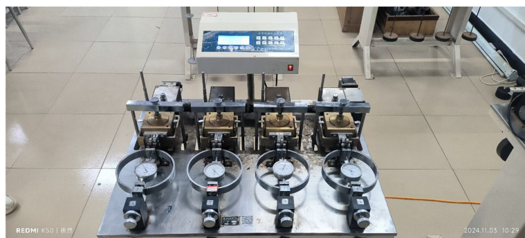
Figure 3. ZJ-type strain-controlled direct shear apparatus.
