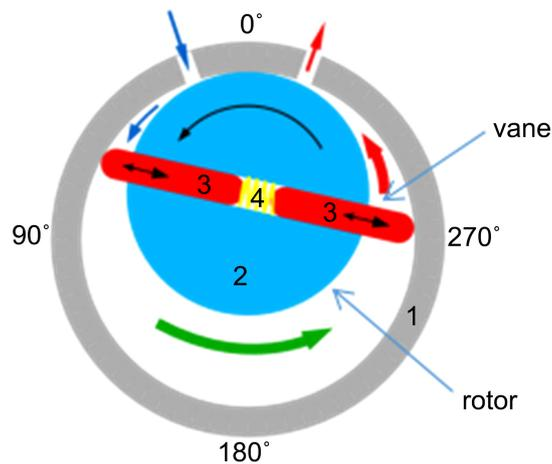
**Figure 7.** The working principle of a rotary vane pump from: (<https://www.cleanpng.com/png-rotary-vane-pump-vacuum-pump-compressor-hydraulic-813040/download-png.html>).
