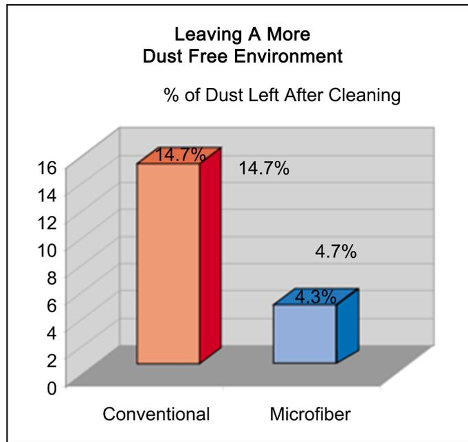
**Figure 11.** The comparison of the ability to collect the dust between conventional materials and microfibers of the working principle of microfibers.
