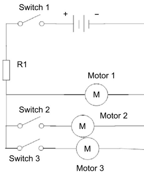
**Figure 6.** The circuit design of the remote-controlled eraser.
