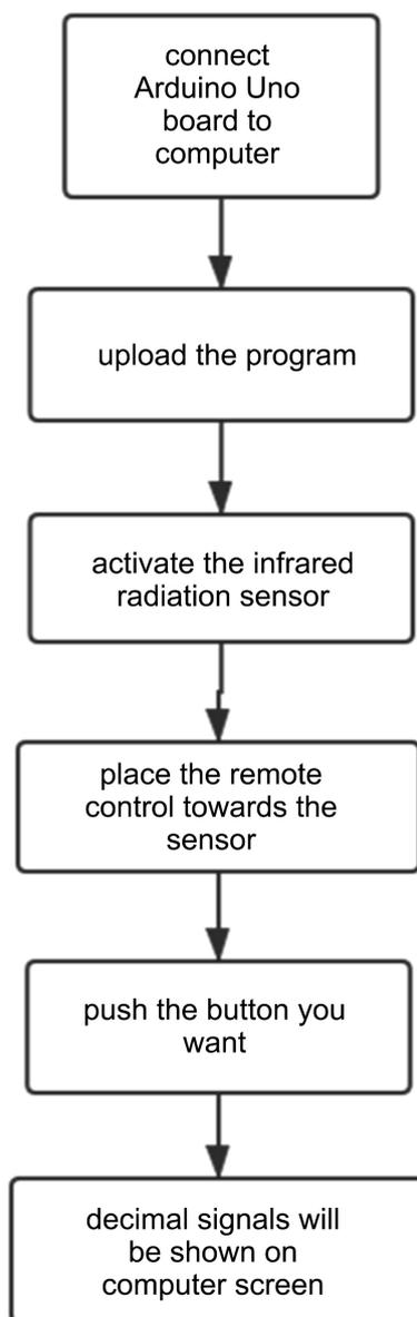
**Figure 4. Flow chart of detecting the infrared signal of different buttons.**
