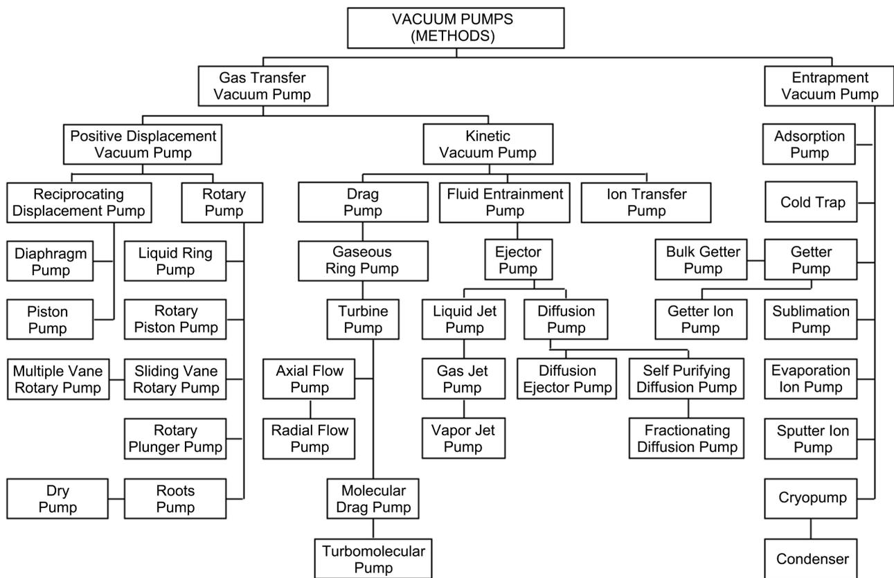
**Figure 8.** Different methods of vacuum pumps.
