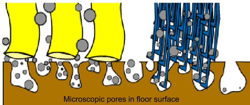
Microfibers physically go into microscopic pores in surfaces to remove dirt, dust & microdust.
