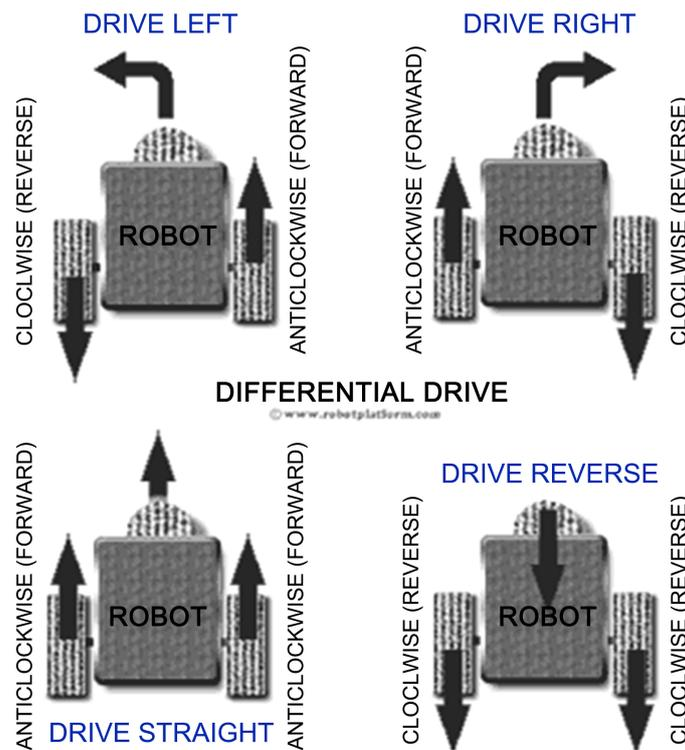
**Figure 12.** The working principle of a differential wheel system (higher rate of rotation at the right wheel will turn the vehicle to the left; higher rate of rotation at the left wheel will turn the vehicle to the right) from: [http://www.robotplatform.com/knowledge/Classification\\_of\\_Robots/wheel\\_control\\_theory.html](http://www.robotplatform.com/knowledge/Classification_of_Robots/wheel_control_theory.html).
