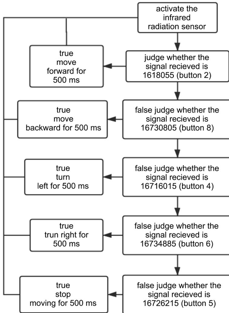
**Figure 5.** The flow chart of the remote-controlled system.
