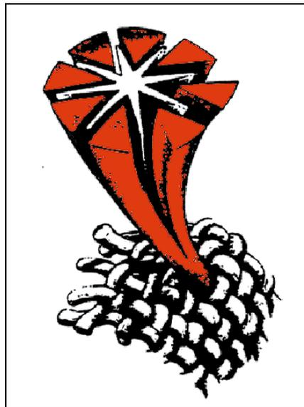
**Figure 9.** The structure of microfibers.
