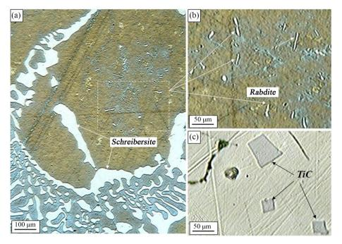
**Figure 5.** Mineral phases of "Ilecta" in reflected light: (a)-(b) eutectic decomposition of gupeiite with schreibersite and needle crystals of rhabdite in gupeiite (structural etching of HCl); (c) crystals of Ti carbide in gupeiite.
