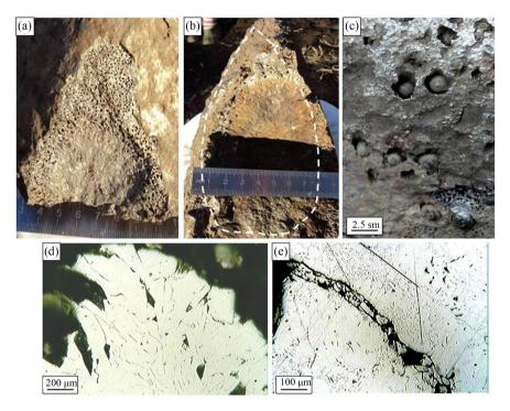
**Figure 4.** Features of the morphology of the gupeite body: (a)-(b) wedge-shaped cross-section of the "Ilekta" sample on the chip (photo of one of the hunters, Gennady Porfirievich.Berzin); (c) bubble surface; plastic (d) and brittle (e) deformations clearly visible on the slice.
