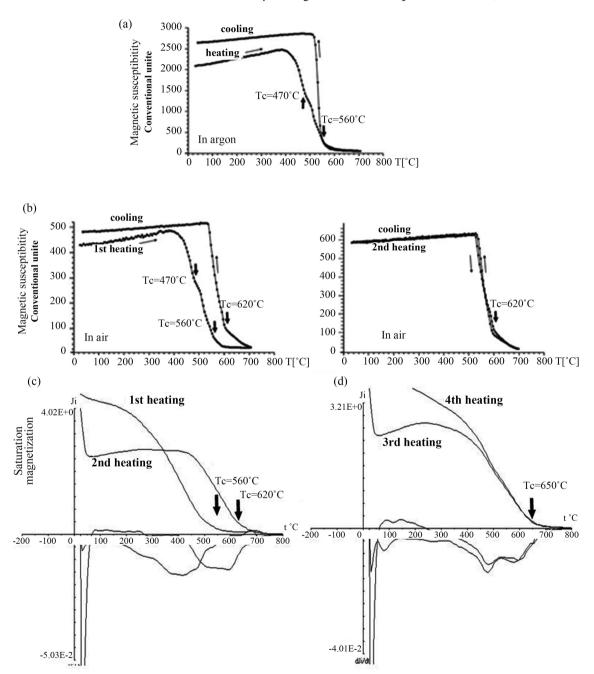
**Figure 7.** Magnetic properties of the Ilekta sample: (a)-(b) thermocappametry curves in argon (a) and air (b): (c) dependence of saturation magnetization on temperature (the lower part of the graphs are differential curves).
