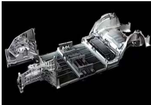
Figure 1. Large Al alloy die-casting underbody.
