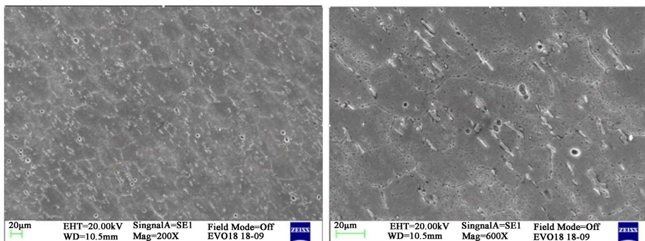
**Figure 2.** Microstructure of 2A70 aluminum alloy.
