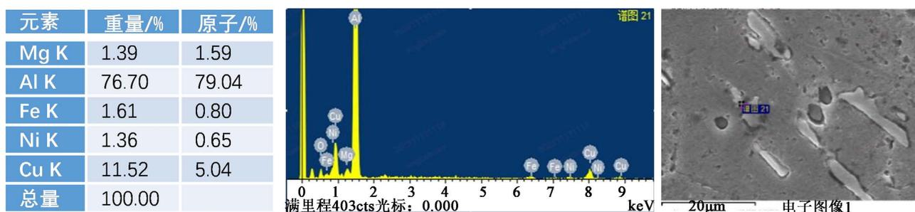
**Figure 5.**  $\text{Al}_2\text{CuMg}$  phase and  $\text{Al}_2\text{CuNi}$  phase of 2A70 aluminum alloy.
