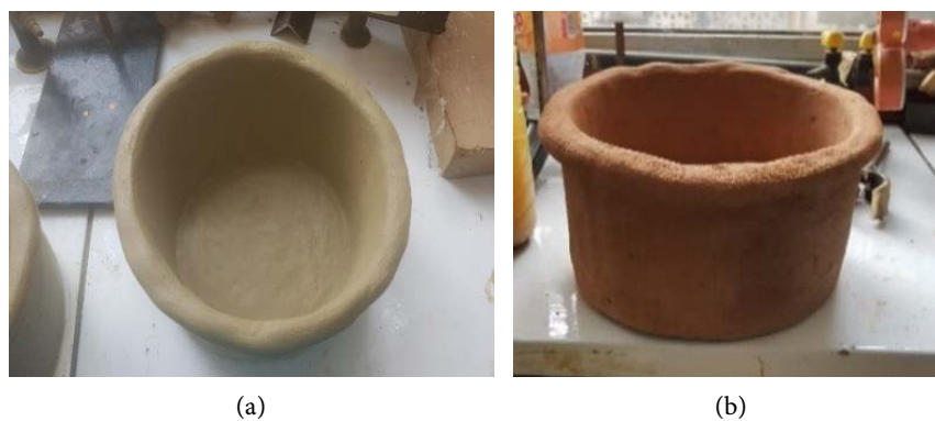
Figure 8. Aspect of the ceramic pot filter (a) before sintering and (b) after sintering.
