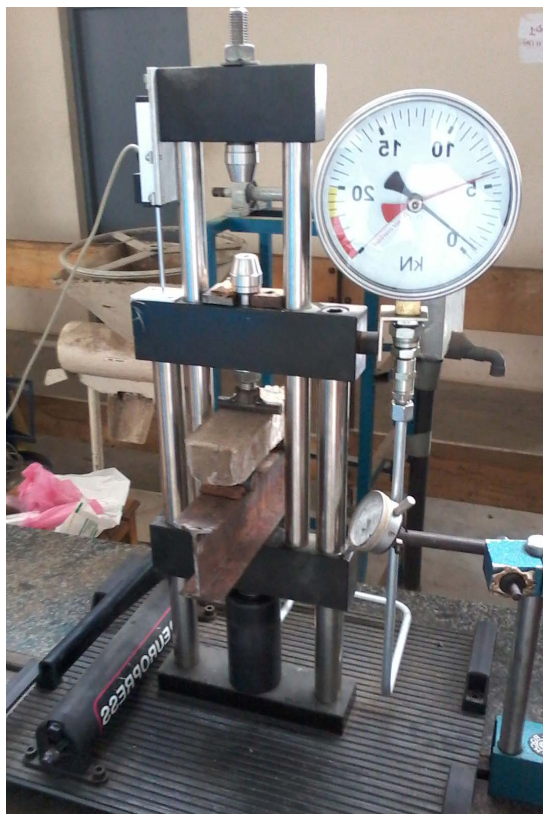
Figure 2. Bending test device.
