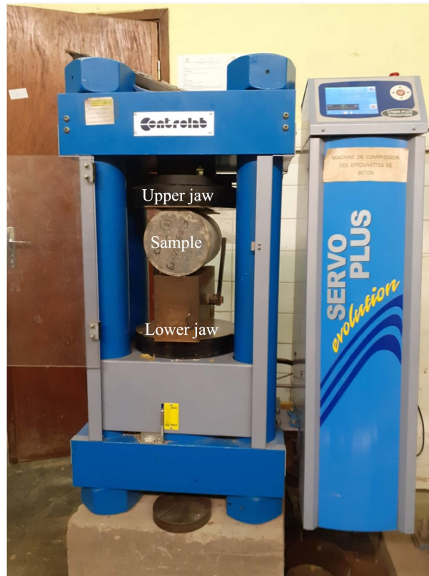
Figure 3. Splitting tensile test and compression machine.
